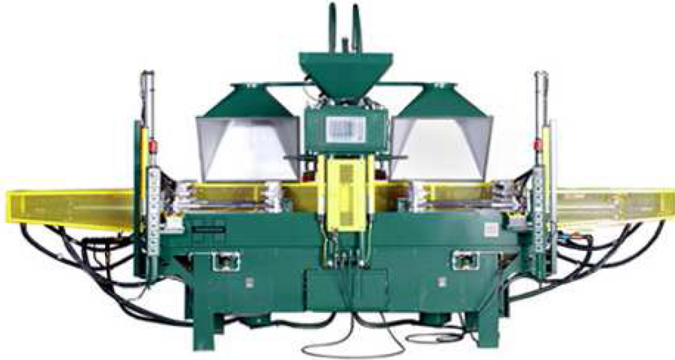
Shell Core Machines-Dual Station
